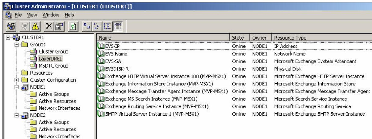
Figure 1: Two Node Windows Server 2003 Cluster with Exchange Server 2003
