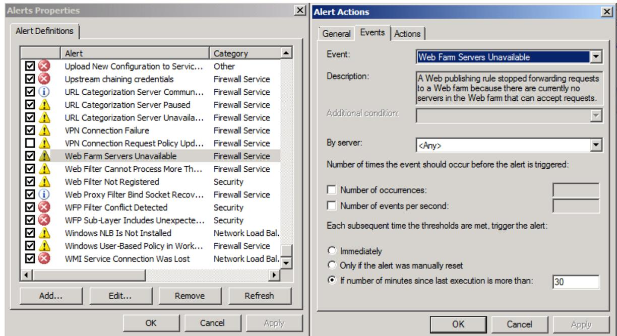
Figure 11: Web Farm monitoring and alerting
