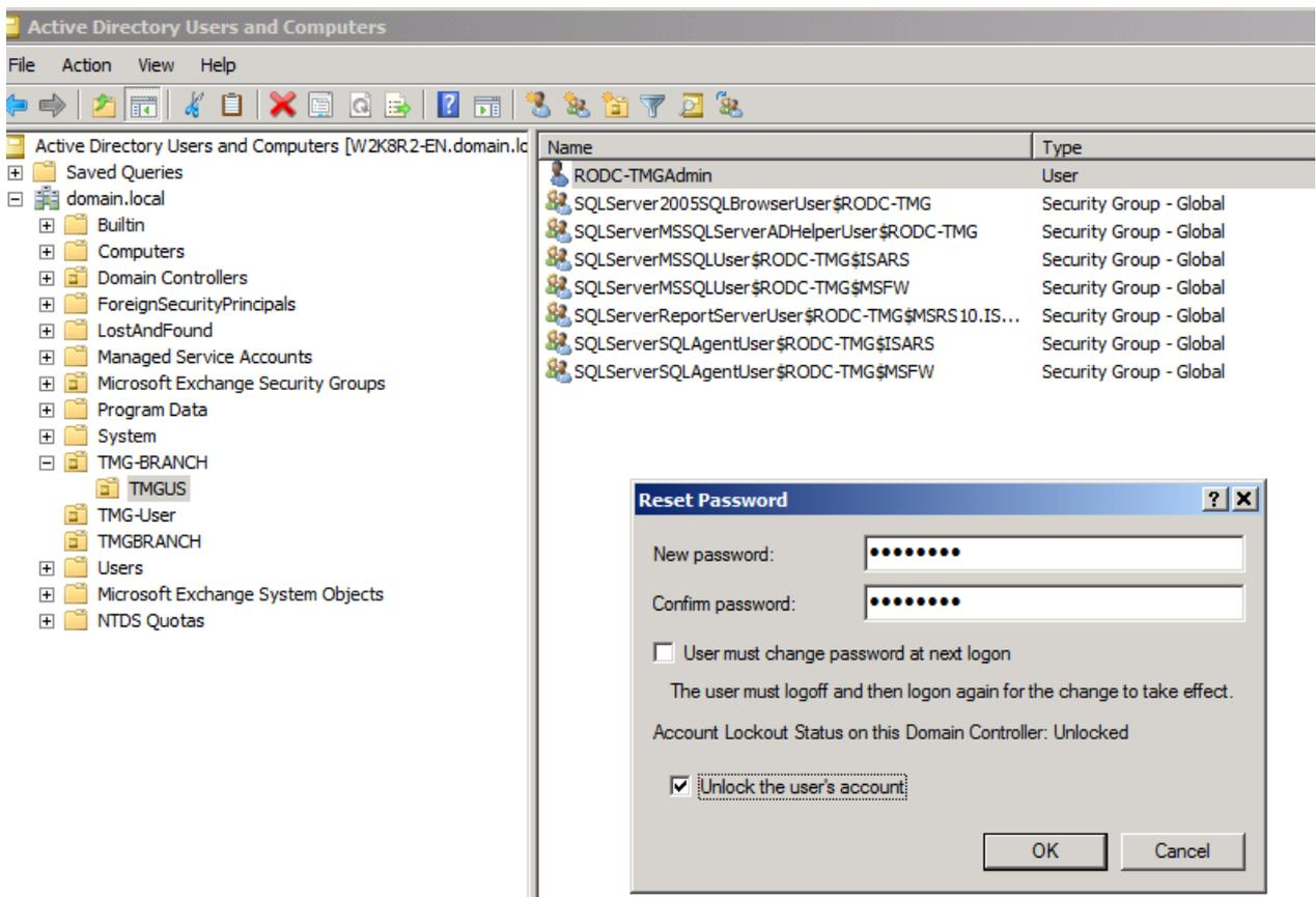
Figure 5: Change the password of the TMG Service account if you doesn't specified one in the script
