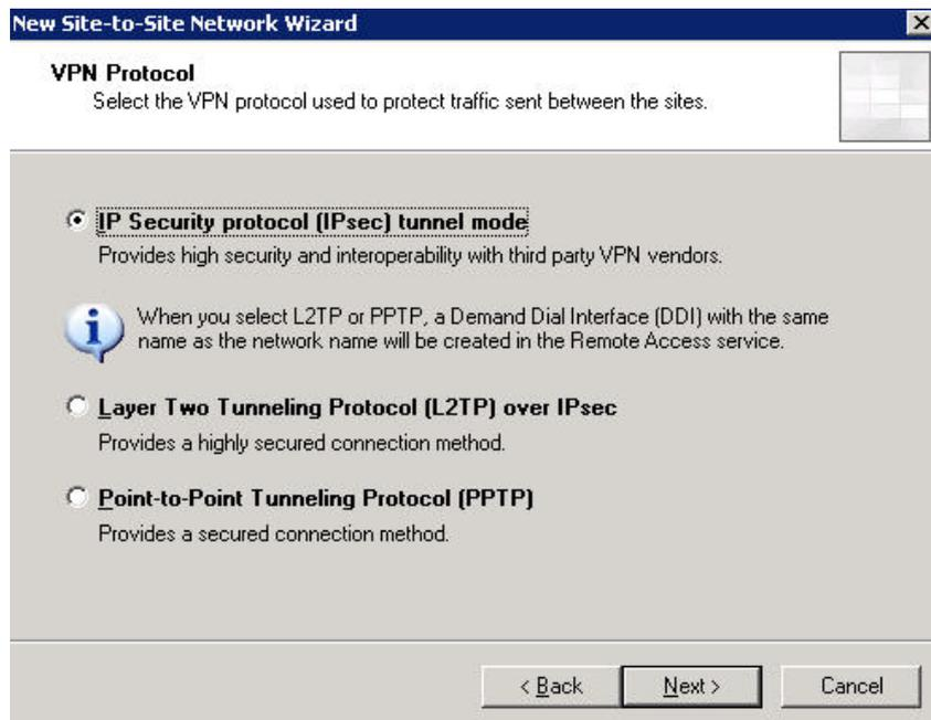
Figure 4: Select IPSEC Tunnel Mode
