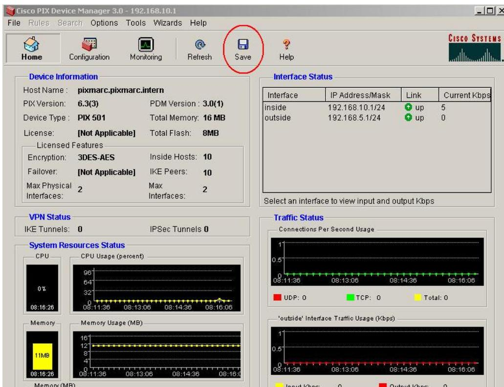
Figure 28: Save configuration in NVRAM
