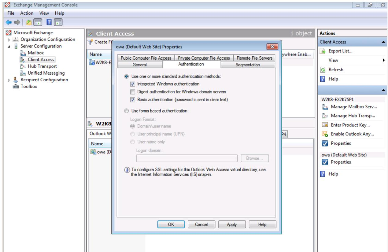
Figure 1: Change authentication from FBA to Basic authentication
