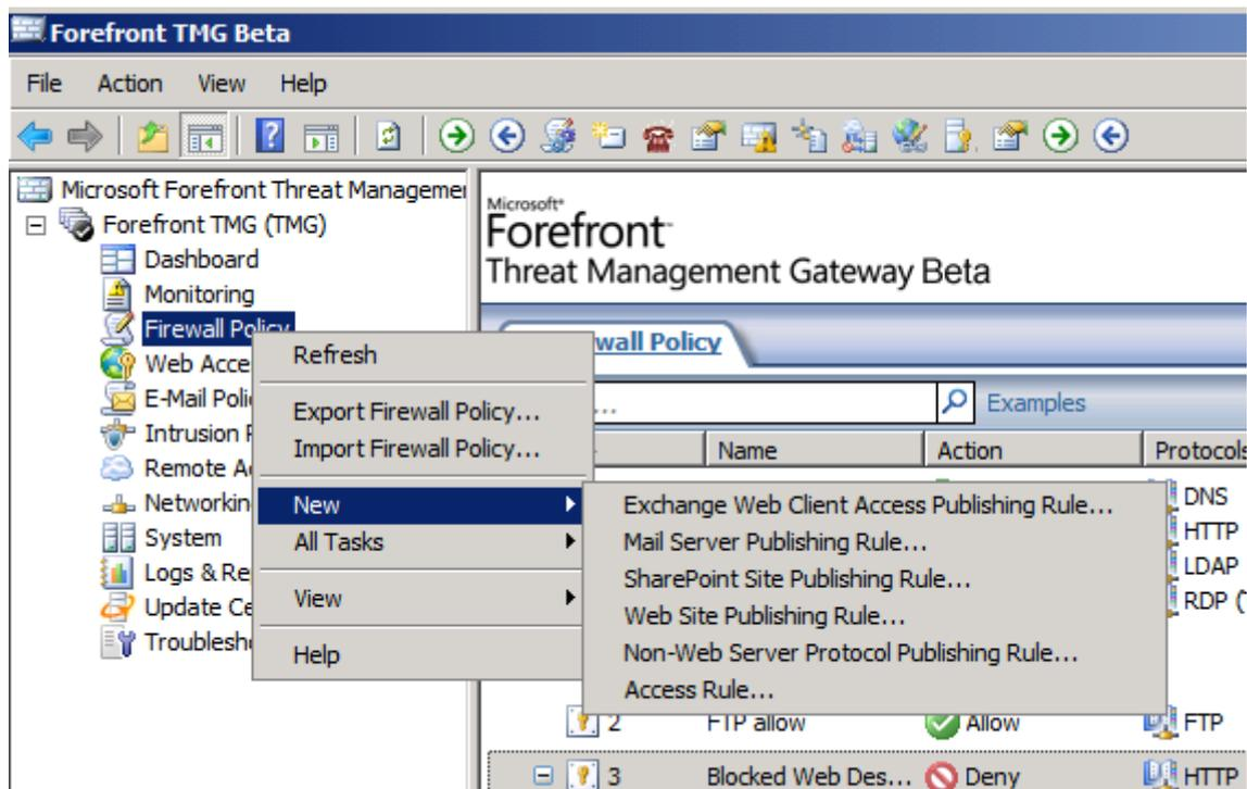
Figure 5: Create a new Exchange Web Client Access Publishing Rule
