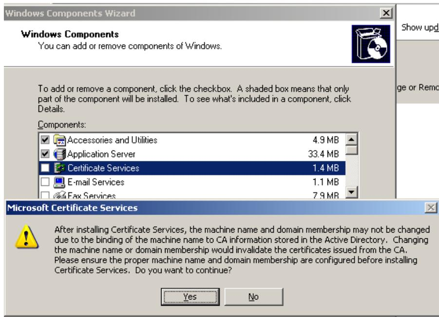
Figure 2: Installing a Windows CA
