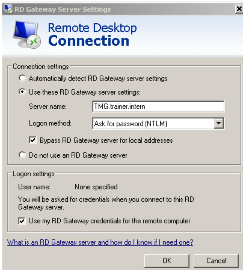
Figure 15: Enter the RD Gateway INTERNAL Server name
