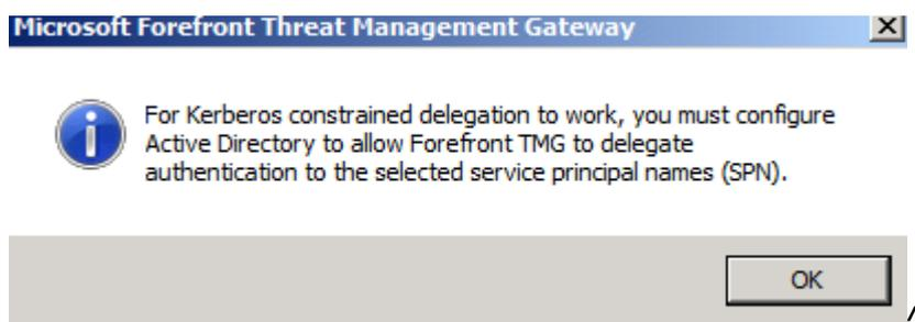
Figure 10: Information message for additional KCD configuration
