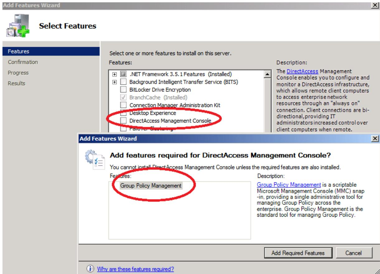
Figure 1: Installing the Windows Server 2008 R2 DirectAccess feature
