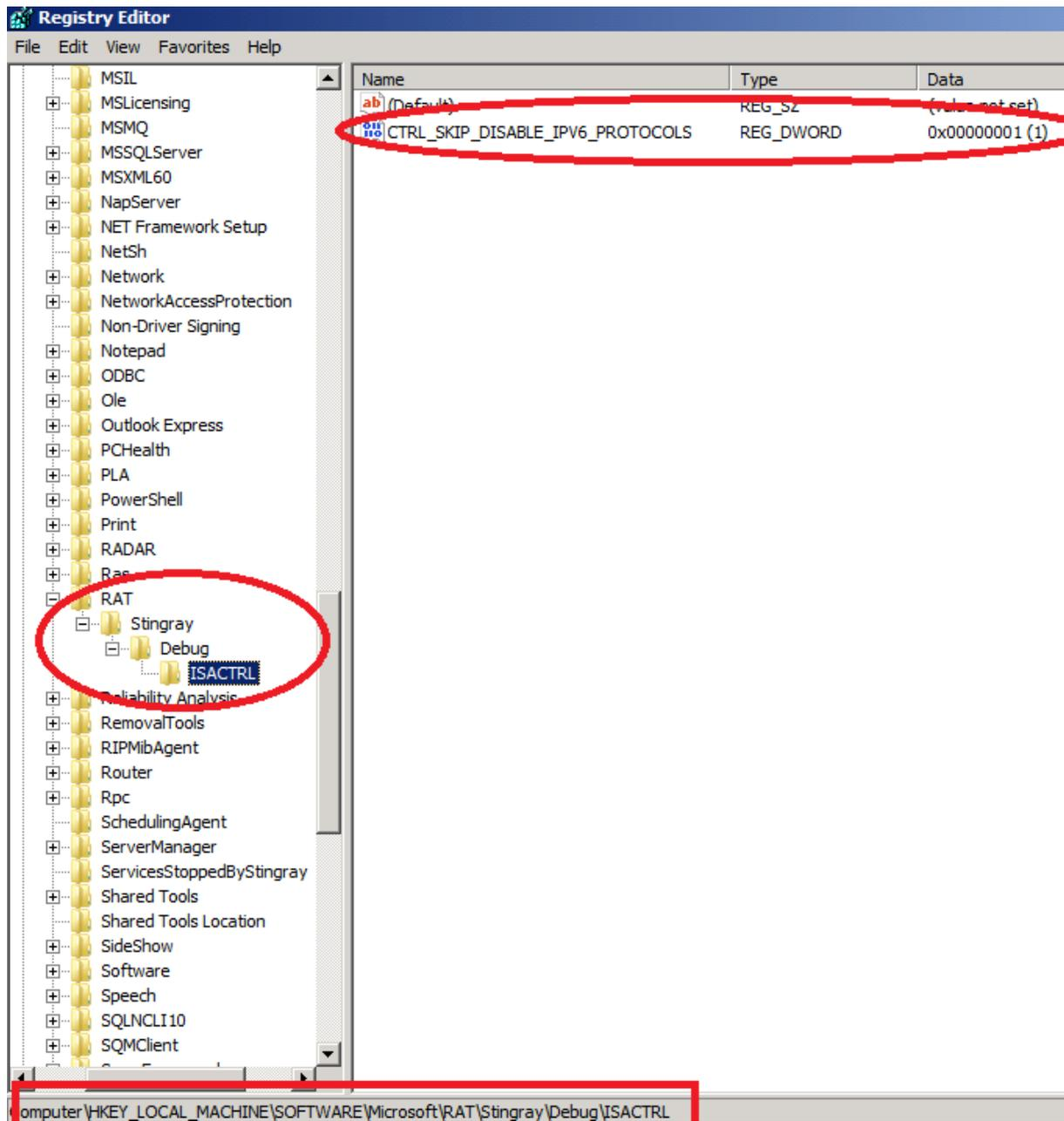
Figure 3: Script to activate Ipv6 protocol support for Forefront TMG
