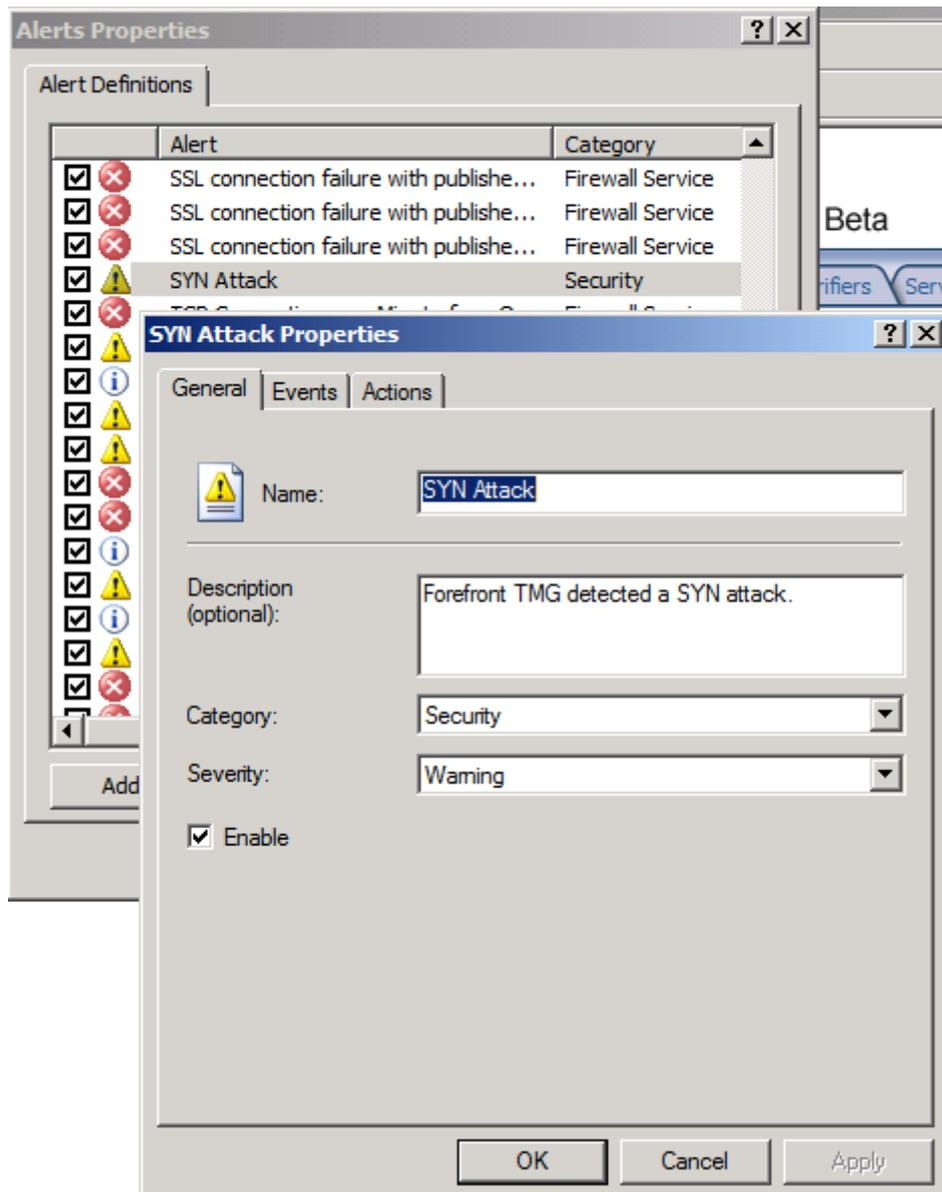
Figure 9: Configure Intrusion detection alerts
