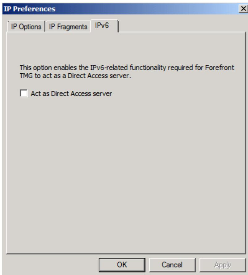
Figure 4: Enabling Direct Access support in Forefront TMG
