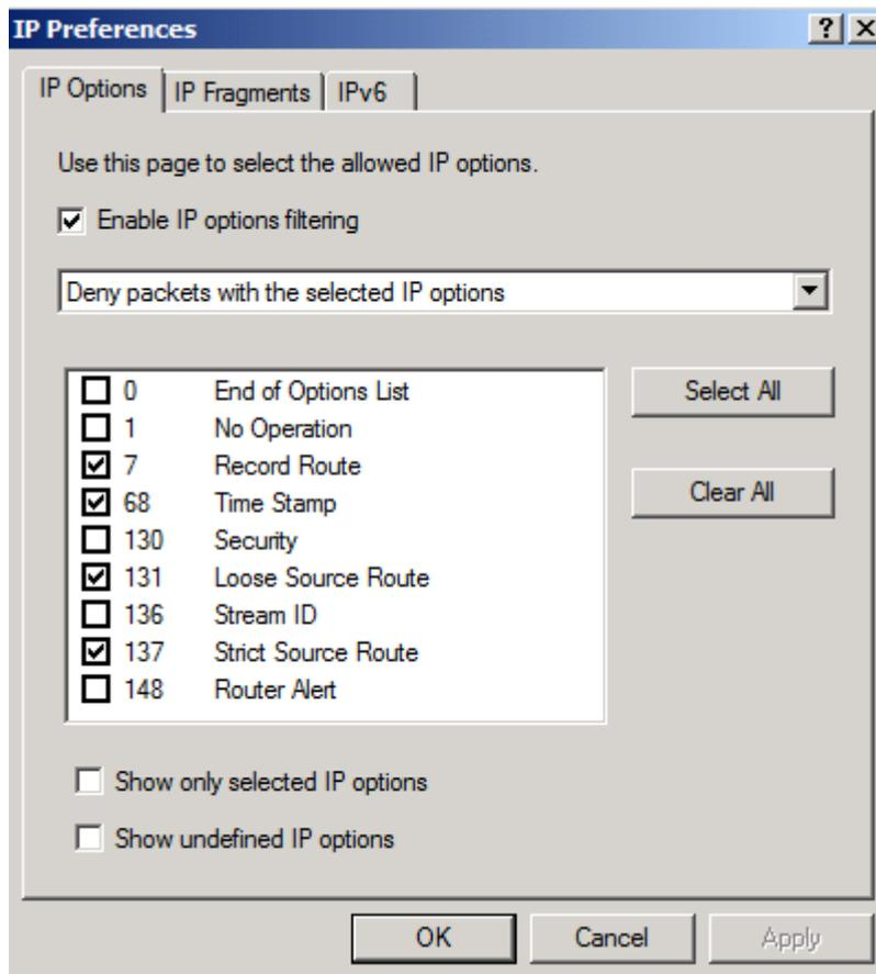
Figure 3: IP options filtering
