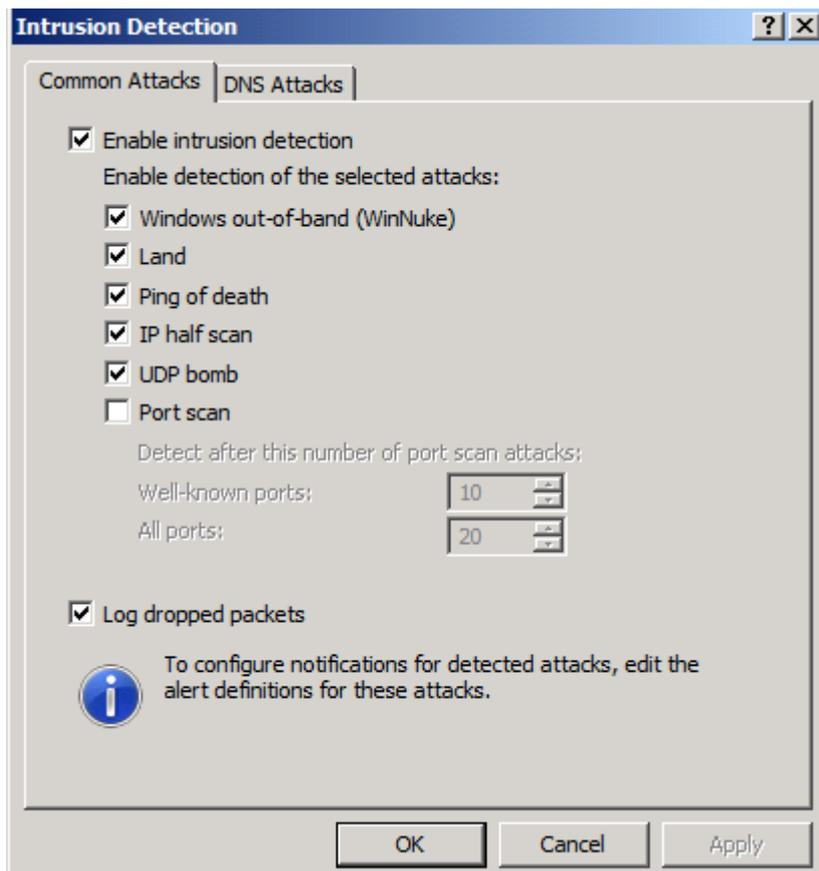
Figure 1: Protecting against Common Attacks
