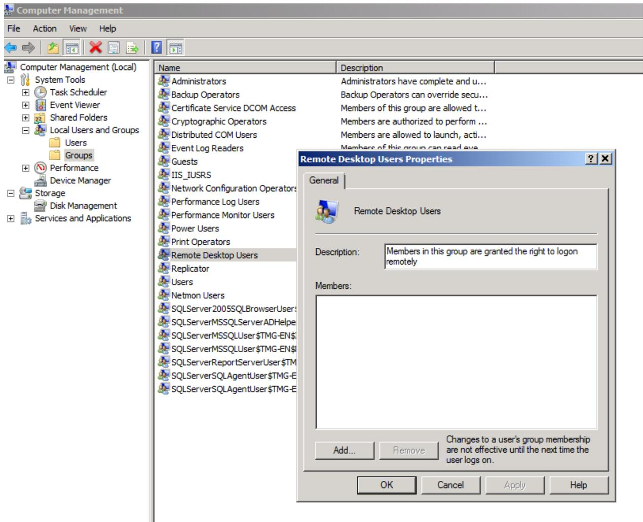
Figure 3: Allow users to access the TMG Server via RDP
