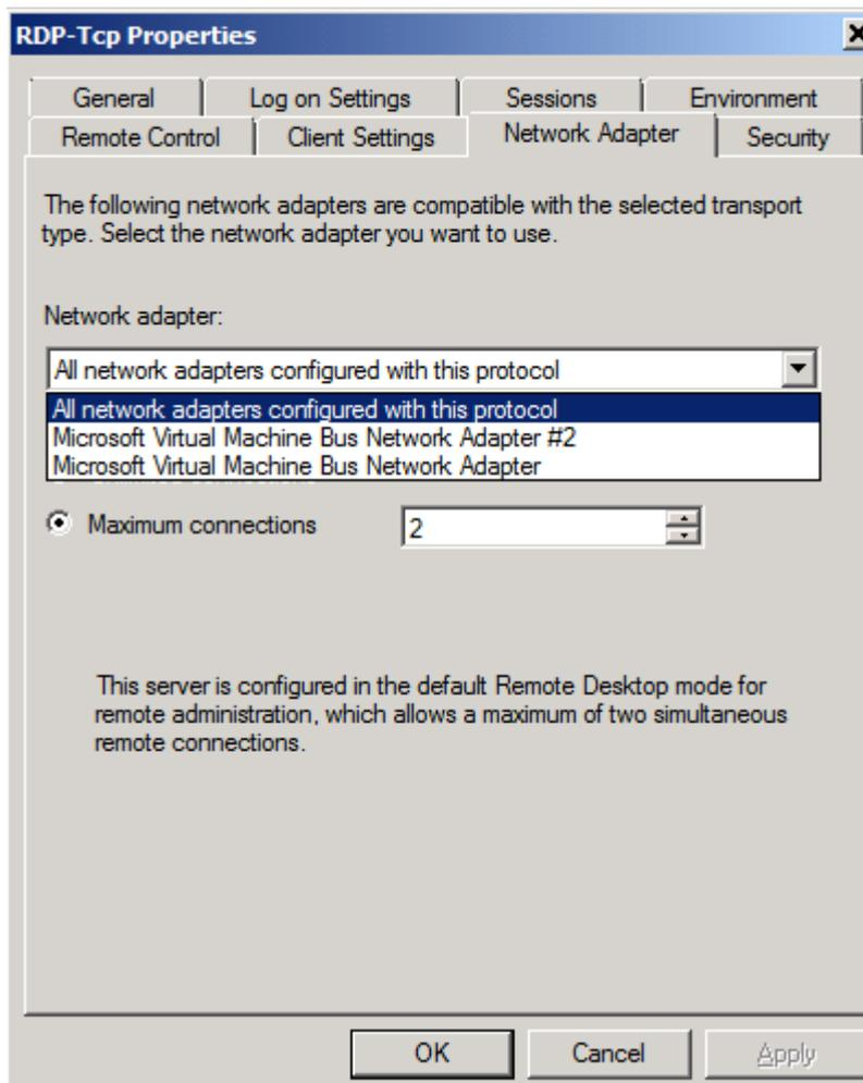
Figure 2: RDP properties – Network adapter
