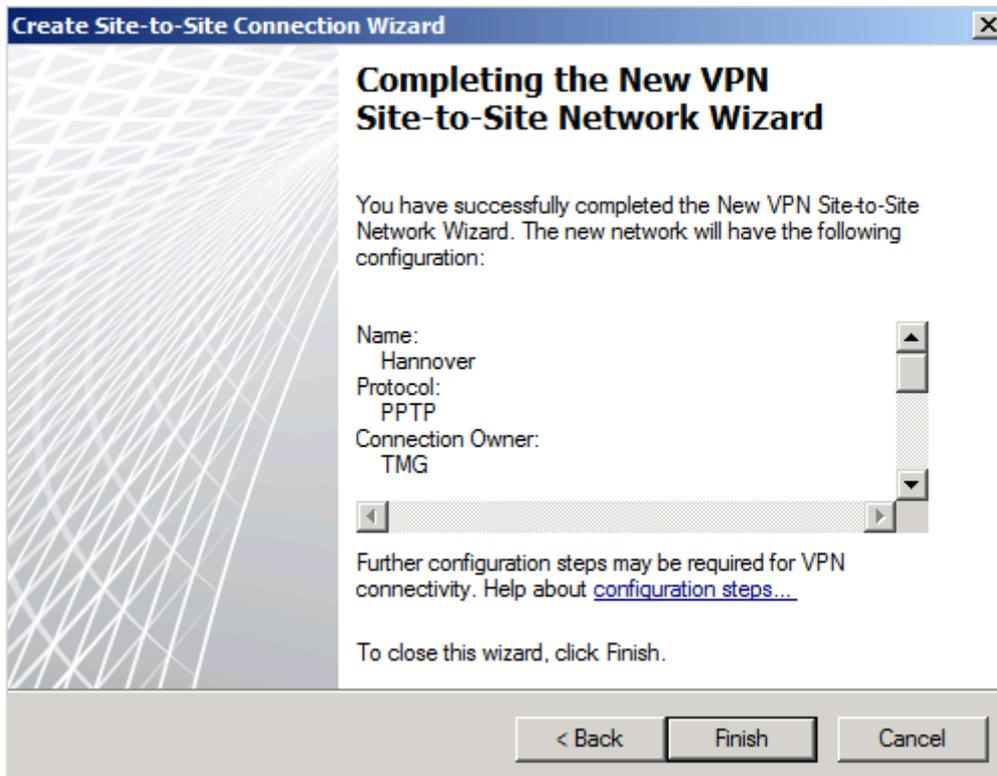
Figure 15: Completing the new VPN Site-to-Site Network Wizard
