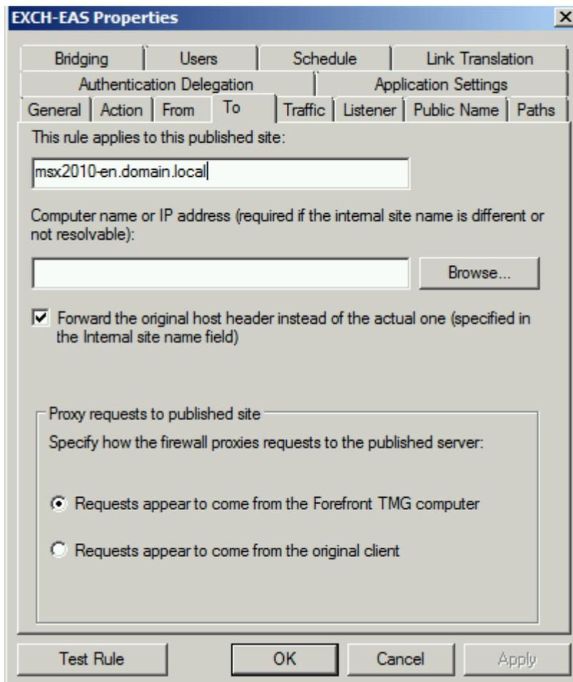
Figure 9: Avoiding error message 500 – Certificate principal name is wrong
