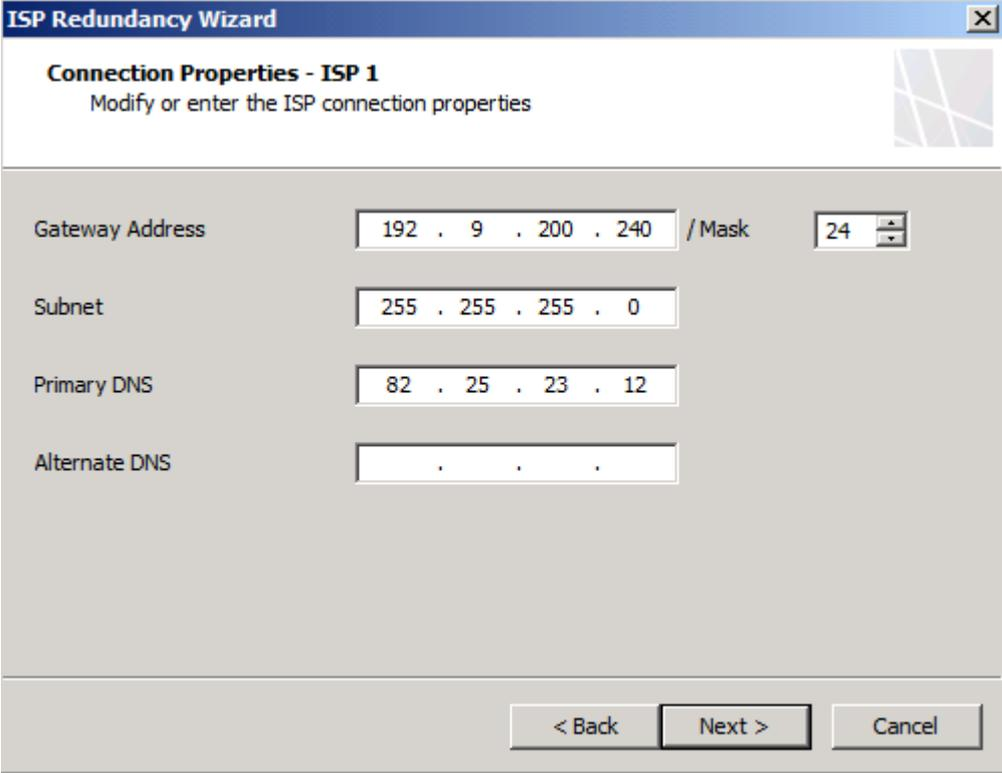
Figure 5: Connection Properties of ISP
