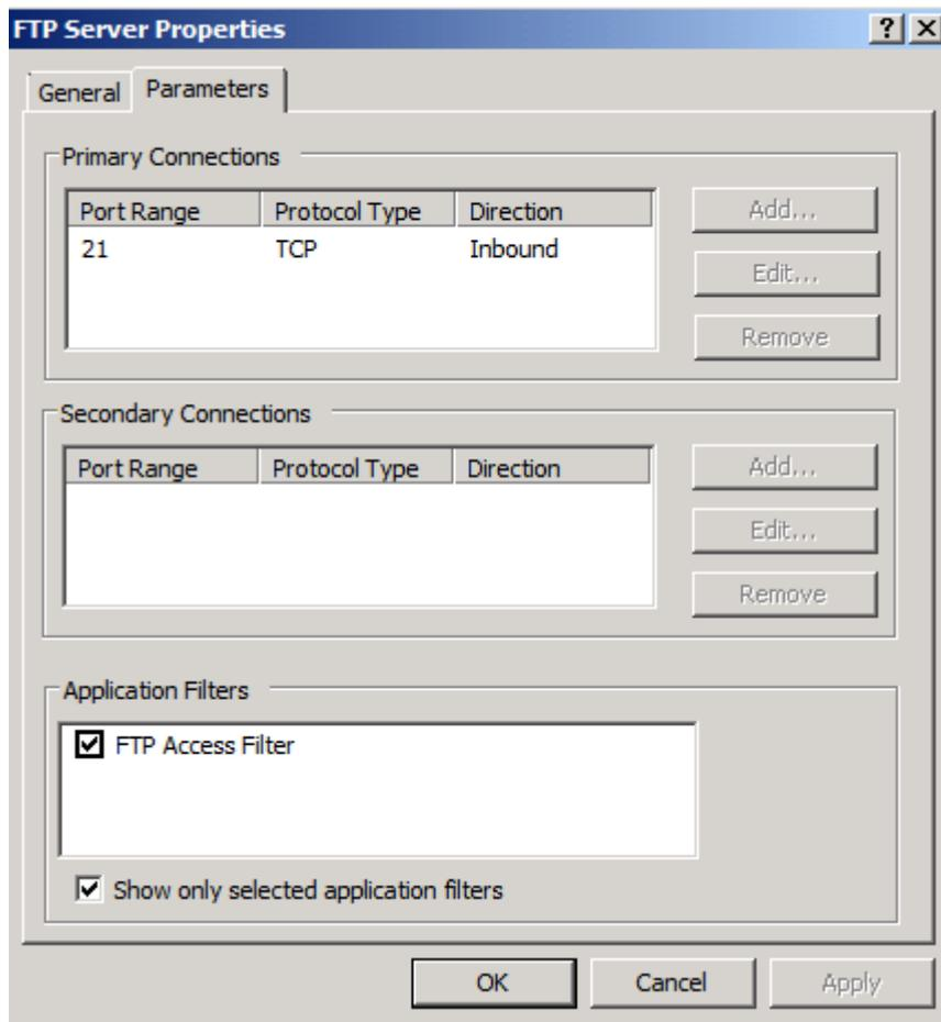
Figure 6: FTP ports and FTP Access Filter binding
